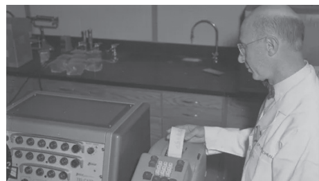
Dr. Meschan checks Tri-Carb liquid scintillation counter used to detect radiation levels.
