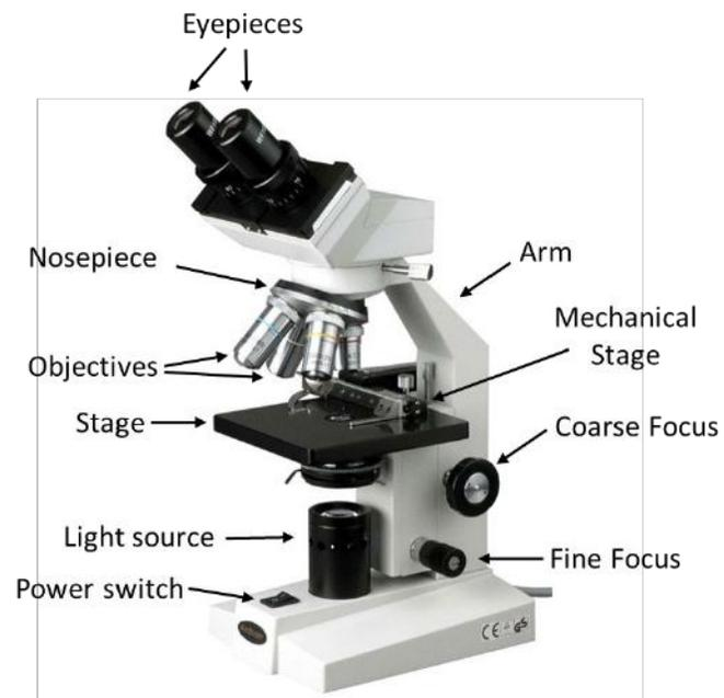
8. Once the cells are in focus, rotate the nosepiece again, so that the 40/0.65 objective is in the back position. There will be very little space between the slide and the objective at this point. Look through the eyepieces and re-focus as needed. Use the fine focus knob at first, and only use the course focus if necessary. Again, if you need to use the course focus knob, be very careful not to the slide touch the objective.
