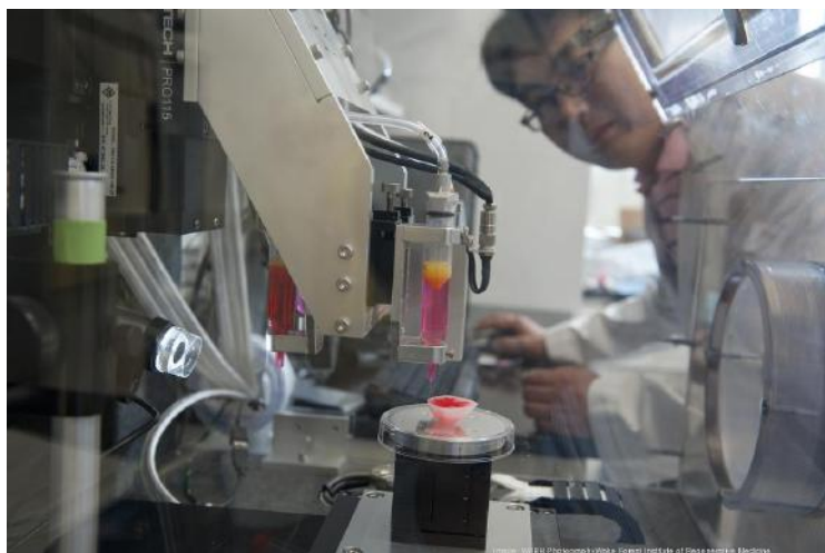
Hyun-Wook Kang, researcher at Wake Forest Institute for Regenerative Medicine (WFIRM) watches as a 3D printer seeds cells onto a kidney scaffold.
